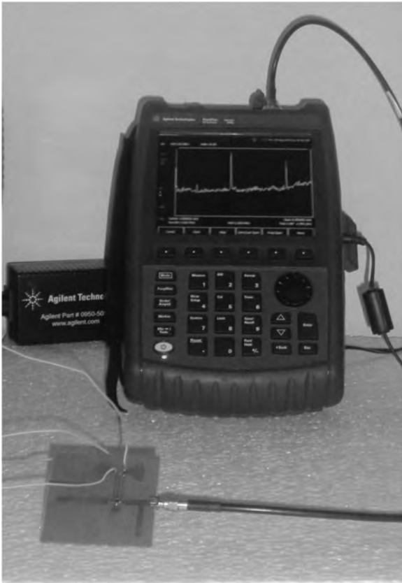
FIGURE 4.21 The oscillator measurement setup. (From Iyer, B., Advances in Intelligent Systems Research , 137, 834–846, 2017 [84].)
